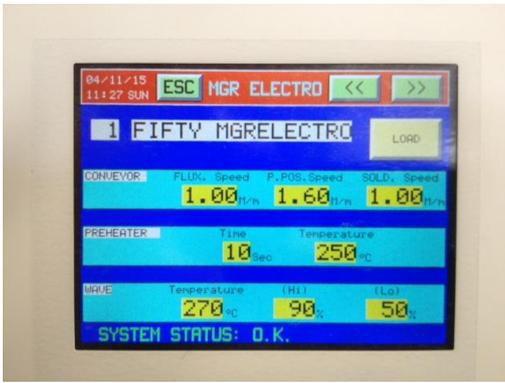
FIFTY is managed by a very practical PLC through which you can set any parameter of the machine. This PLC may recall up to 20 stored programs.
