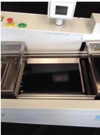
Preheating is performed by an IR panel protected by a PYREX glass and through the PLC the circuit board to be soldered can be stationary in the preheating zone for up to 90 seconds or run in continuous mode for faster production.
